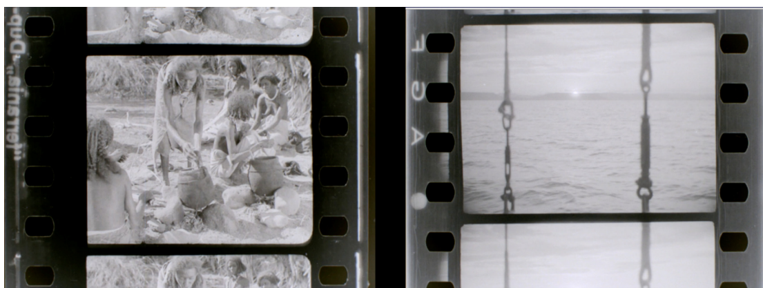
Figure 13 - On the left, one of the frames extracted from the reel 1 reprinted on a sound film “ferrania” Dup and on the right, the reference for the producer’s edge mark AGFA plus a circle.
